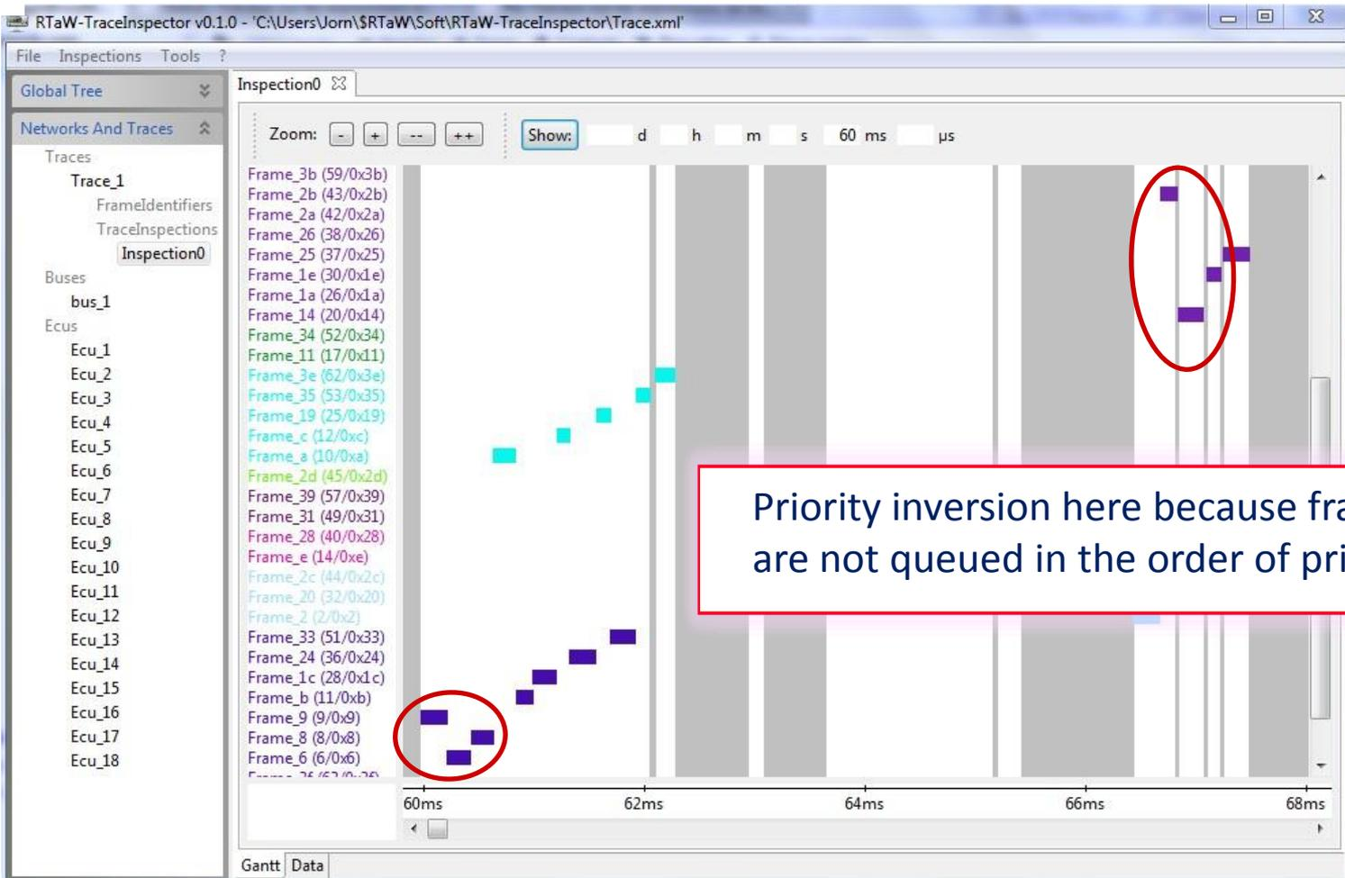
Check comm. stack implementation, periods, offsets, jitters, model for aperiodic traffic and transmission errors, clock drifts, etc .. [RTaW-Trace Inspector screenshot]
