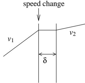
Fig. 12. The amount of work done during a speed change in a typical synchronous circuit is nil.
