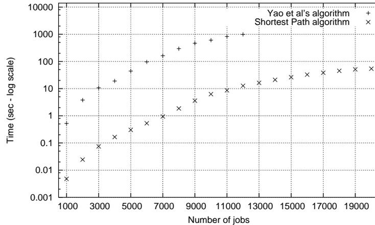
Fig. 6. Computation times of the optimal voltage schedule for the Shortest Path and Yao et al algorithms on the same random sets of tasks. For each problem size, the result is the average of 20 experiments. Computations were stopped when at least one experiment took more than one hour of CPU time.
