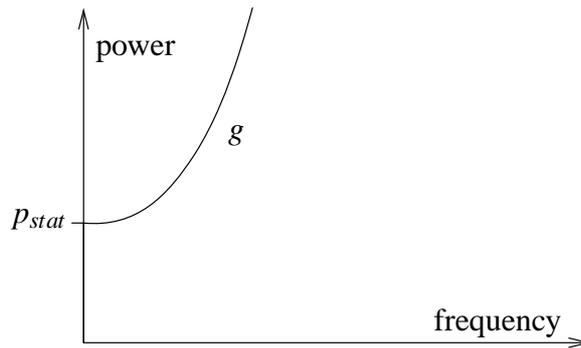
Fig. 15. Example of a non-convex energy consumption function. The energy consumed at frequency 0 is not nil due to the static power.
