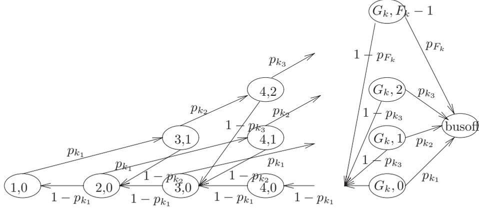
Fig. 7. Markov chain where  $\beta = 1$ ,  $\alpha_1 = 2$  and  $\alpha_2 = 1$ . The value of  $G_k$  is  $\sum_{j=1, \dots, F_k-1} \alpha_j$ .
