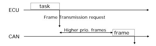
In addition, avoiding consecutive frame constructions on an ECU allows to reduce latency
